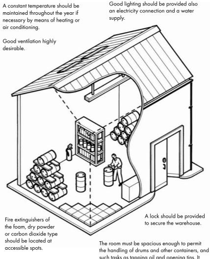
The room must be dust-free, accordingly it should be tiled or treated with a suitable paint.
