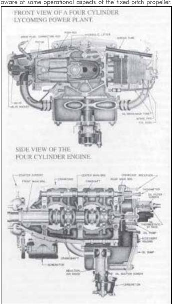
Cutaway of a Four-cylinder Power Plant
