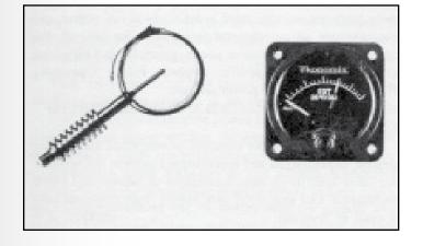
The simple gauge shown in the illustration is quite satisfactory for the less complex engines. An advantage of the EGT over the cylinder head temperature gauge is one of an almost immediate response to EGT Probe and Gauge
