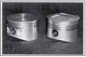
Although we can create a more efficient engine by increasing the compression ratio, there are limits and a compromise is needed. If the pressure is too high, preignition will occur and produce overheating. Compression ratio is a controlling factor in the maximum horsepower developed by an engine, but it is limited by present-day fuel grades and the high engine speeds and manifold pressures required for takeoff.
