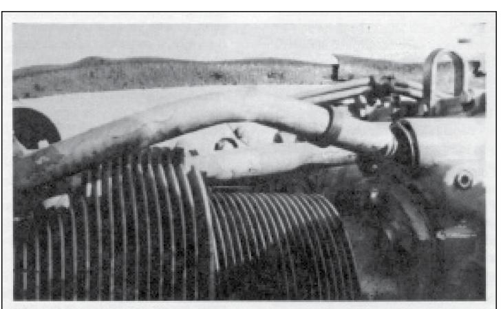
When indications of value sticking are neglected, a best pashood and damaged shroud tube may result. In the picture above, note the severe bend in the normally straight shroud tube.
